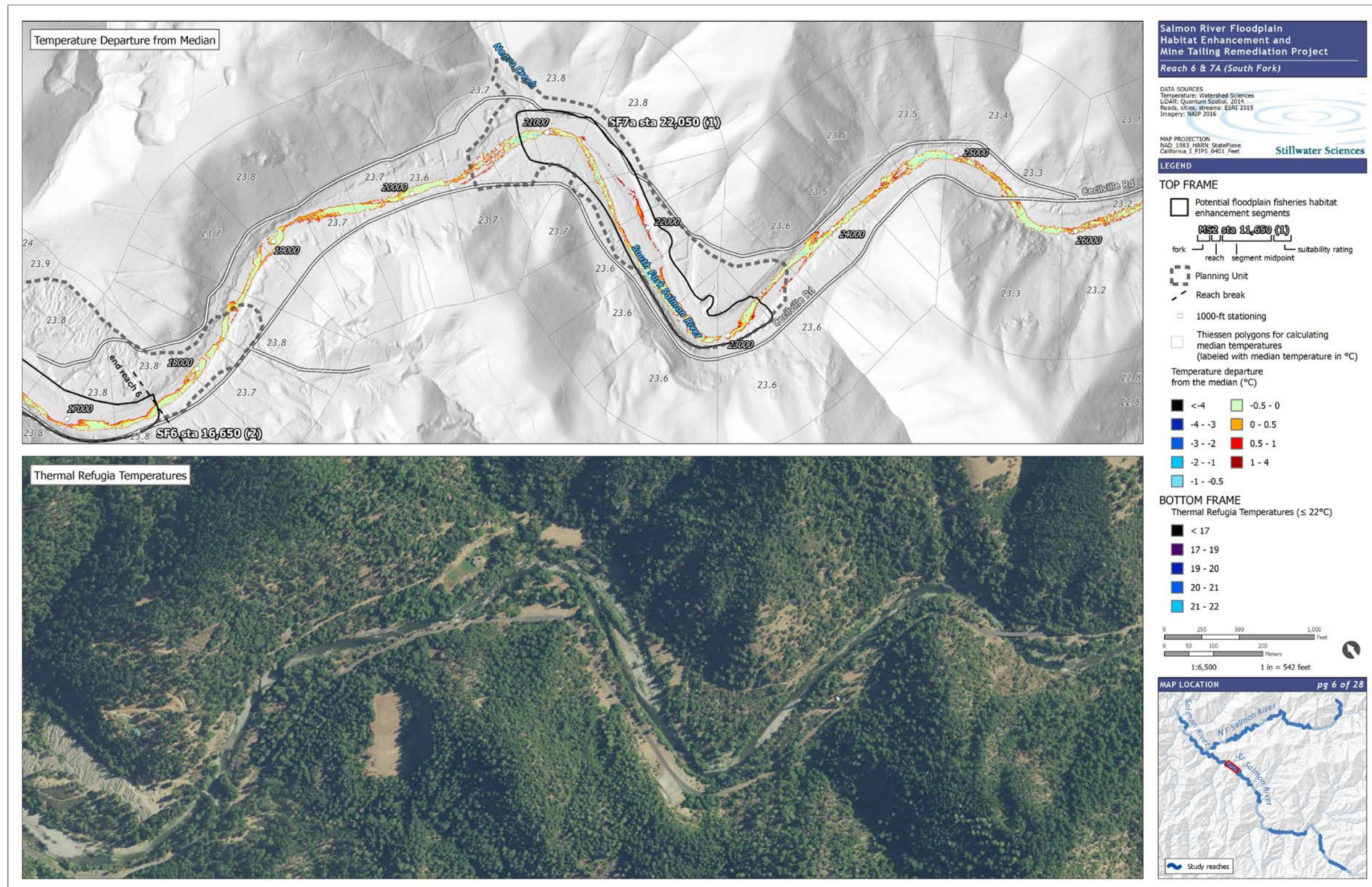
Figure A-11. Thermally suitable habitat and localized thermal refuges in predominantly alluvial reaches within the Salmon River project area based on 2009 TIR data, Tile 6 of 28.
