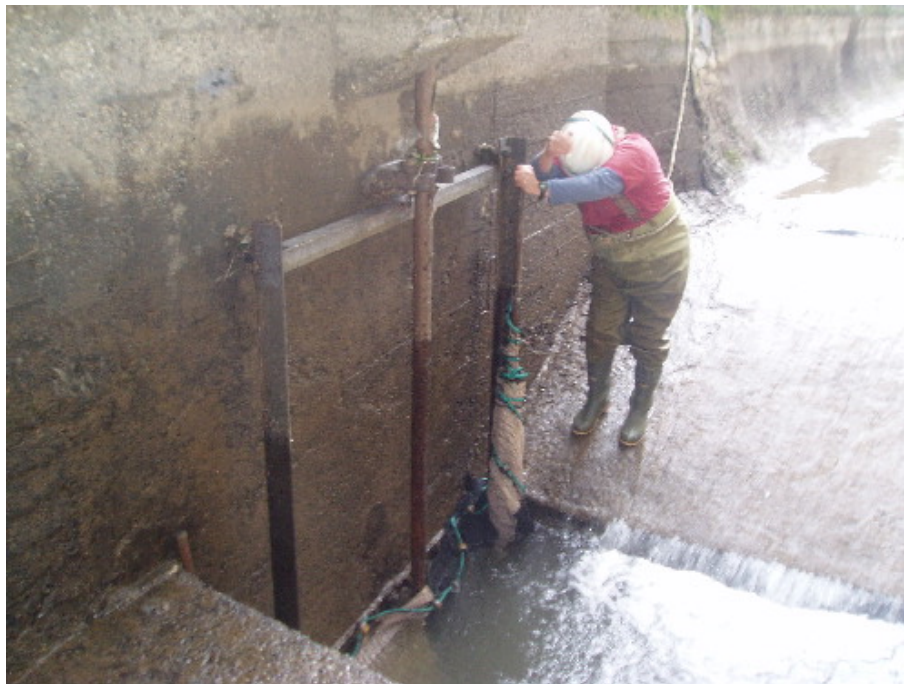
FIGURE 3. Seine nets were placed across the spill gates of larger sediment traps during drawdown to prevent the loss of any fish prior to electrofishing.
