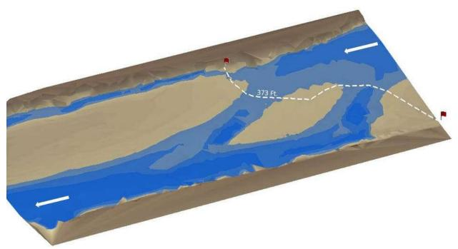
Figure 7. Riffle 96 shallowest course from bank to bank over site topography.
