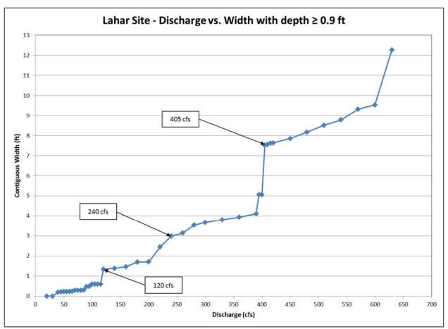
Figure 8. Lahar Site – Discharge versus width with depth ≥ 0.9 feet
