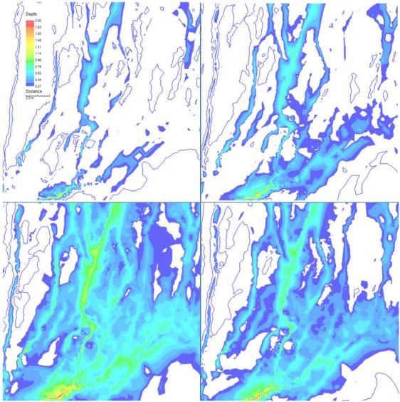
Figure 9. Depth profiles in the limiting choke point area of the Lahar site. Flow levels start at the upper left with 40 cfs and move clockwise around to 120, 240, and 405 cfs.
