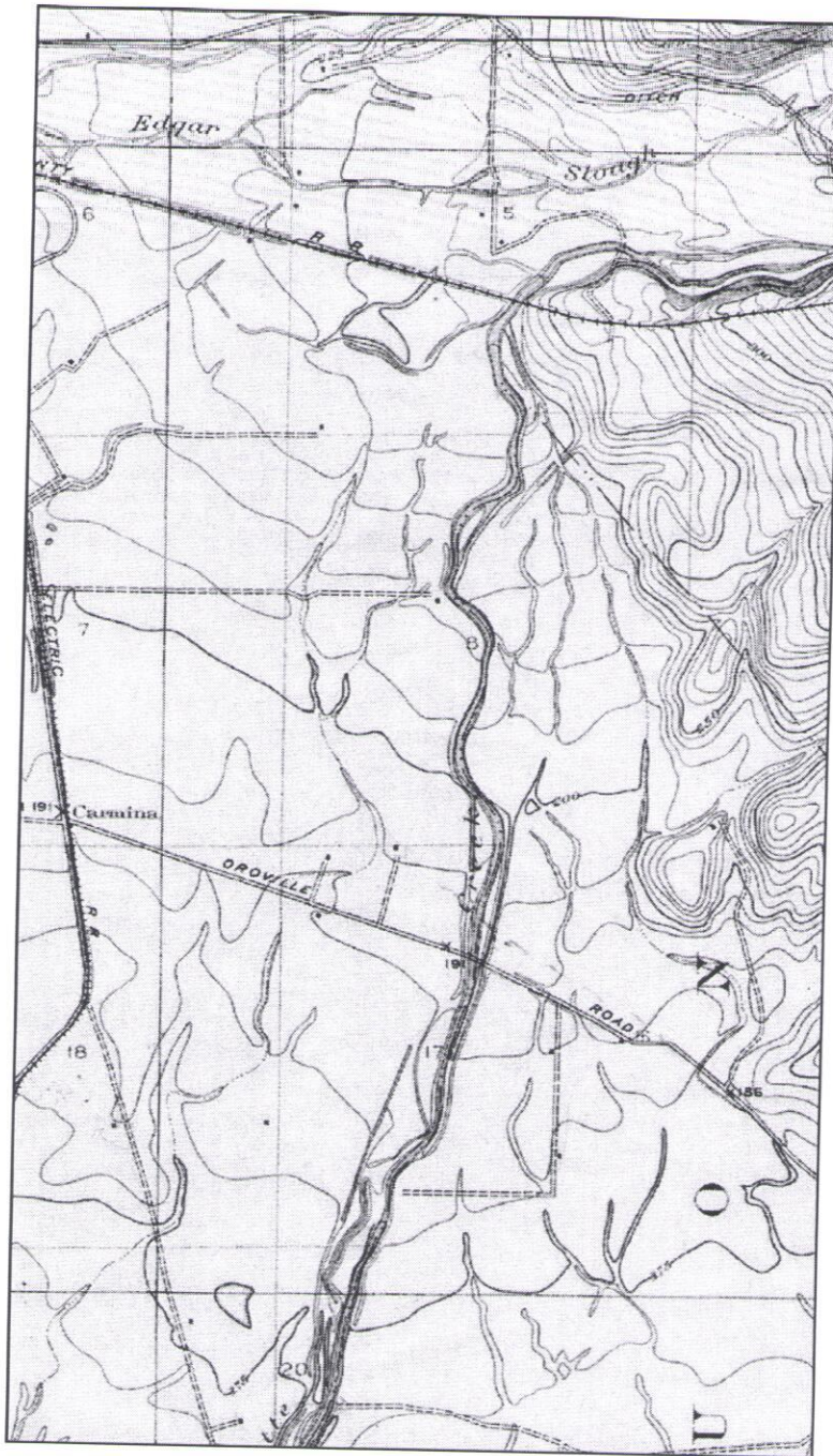
Figure 3-6. A portion of the USGS Durham Quadrangle, based on surveys in 1910. The contour interval is five feet. Highway 99 now crosses the creek just downstream from the island (about a third of the way down the figure, just north-east of a symbol marking a structure at the end of an east-west trending road), approximately parallel to the dash-dotted line which is the boundary of the Esquon Rancho. Note the break in the levee on the left bank just upstream from the island, and the relict leading from it. Only a trace remains of the distributary Little Butte Creek, leaving the channel from the right bank.
